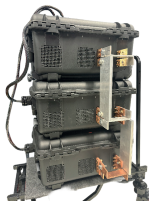
Series Connection with 2 boosters
