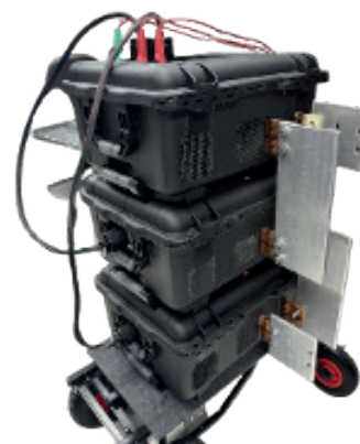
Parallel Connection with 2 boosters
